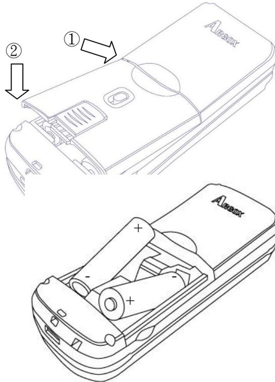
4. Make sure cover is closed and slide two latches back.
