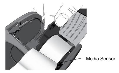
4. Install the Media Shield into Media Compartment, and lean closely against the media supply roll:
