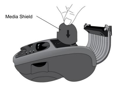
Pull a short length of media out of the printer. Close the Media Cover and press until you hear a click, to properly latch:
