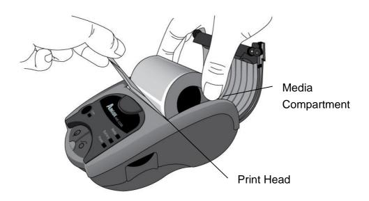
For media supply rolls with width less than 3 inches:
