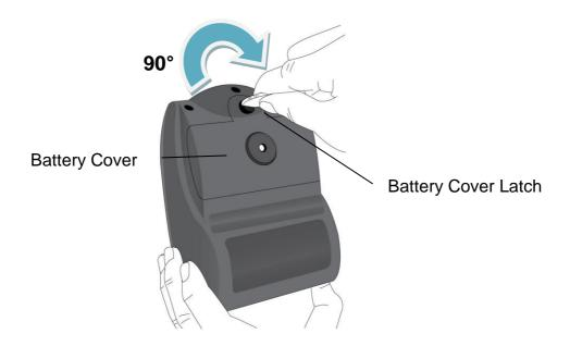
2. Remove the Battery Cover and install the Battery Pack into the
