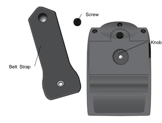
2. Attach the Belt Strap onto the Knob.
