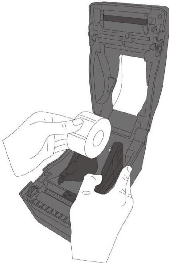
3. Pull the media until it reaches out of the printer. Thread the media under the media guides.
