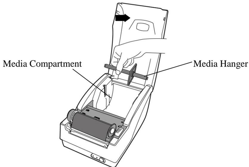
3. Load the media roll onto the hanger from left to right.
