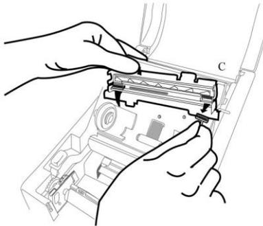
6. Disassemble the print head and the mounting bracket by releasing screws.
