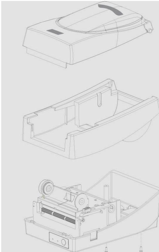
4. Remove the whole print head assembly by releasing the 4 screws at its feet.
