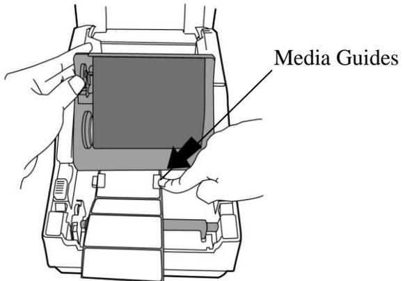
10. Put the print head module down and press down firmly until you hear a snap.
