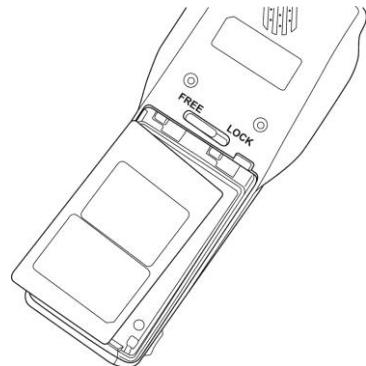
Figure 2-8-2 Installing /Replacing The Battery Pack
