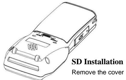
Figure 3-2 Installing SD Card
