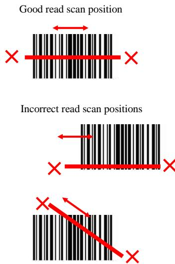
Figure 4-4 Scan Test
