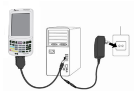
Figure 2-14 Communication through Cable
